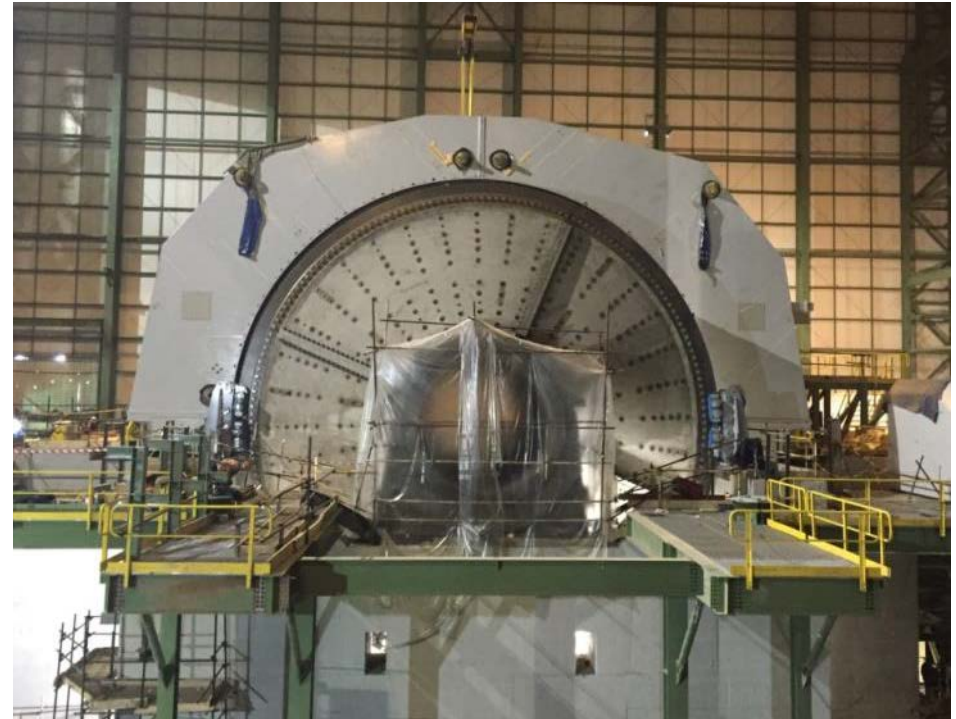
SAG mill with stator
